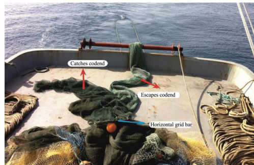
Figure 3. Sorting grid fixed bottom trawl net used in the study
