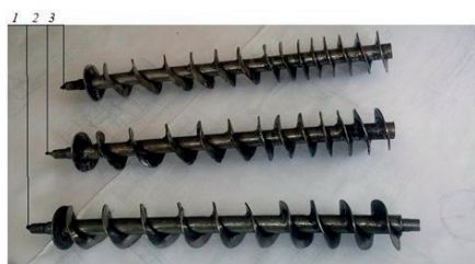
Figure 3. A set of augers with a variable pitch in the sections: 1 - a screw with a pitch change of 20 mm, at t_0 = 0.06 m; 2 - auger with a step change of 15 mm, at t_0 = 0.06 m; 3 - auger with a step change of 10 mm, at t_0 = 0.06 m
