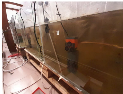
Figure 10. Method of filtering and heating aquariums (original)
