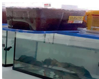
Figure 1. Recirculation aquaculture system (RAS) used in the study and compartments with expanded clay aggregates as biofiltration substrates. The water circulated through an overflow in the biofiltration compartment and returned through a submersible pump
